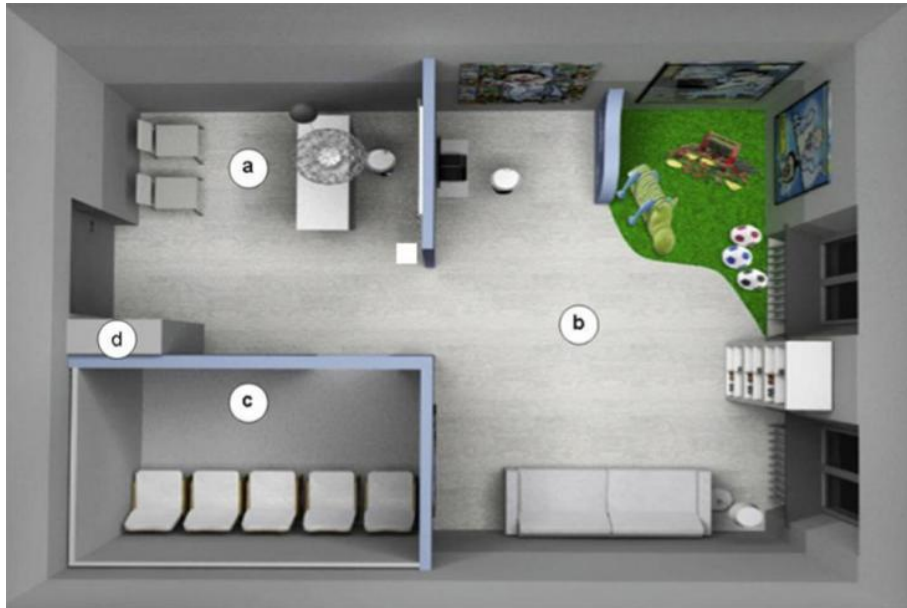
Fig.1. “Salt Clinic”. 3D design: reception/welcome area (a); waiting room with children’s recreation area (b); “Aerosall” halotherapy room (c). ENT Care Unit (d). Cabinet containing the Dry Salt Aerosol Generator – University General Hospital – Bari (Italy).
